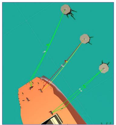
You can also check the fender contacts, shown as a percentage of the fender in contact with the ship's hull.
