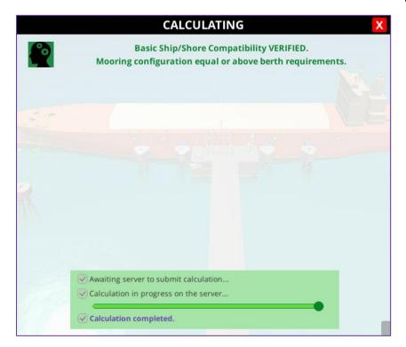
Note that if the mooring configuration does not meet any terminal requirements for number of lines, it will not prevent you from running a calculation but will show a warning and ask if you wish to proceed.
